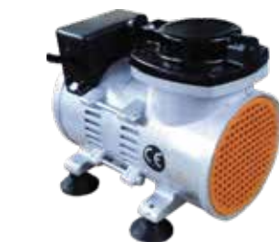
Vacuum Pump Model PCI-15 Max. Flow - 15 LPM, Vaccum - 22" Hg (554 mm) Max. Pressure - 25 Psig, 1/20 HP
